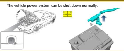
Power off and disconnect the negative cable of 12V low-voltage battery.
