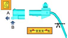
Open the bonnet, pull out the clip from the manual service disconnect(A), press the end of the clip (B) and remove the manual service disconnect. If the situation is very urgent and you cannot disconnect the manual service device, you can simply cut the manual service disconnect harness.
